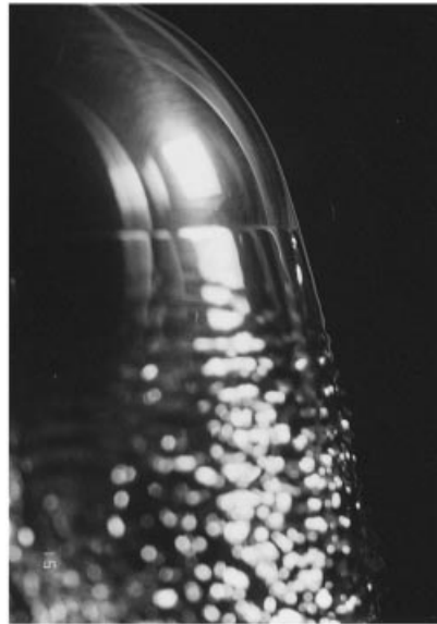
FIGURE 6. A side view of the cavity detachment region with associated dye visualization on the brass sphere. The surface of the cavity forms a sharp curve as it detaches from the solid surface indicating a hydrophilic surface.
